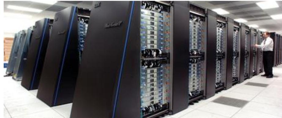
The [IBM Blue Gene/P](#) supercomputer "Intrepid" at [Argonne National Laboratory](#) runs 164,000 processor cores in 40 racks/cabinets connected by a high-speed 3-D torus network.
